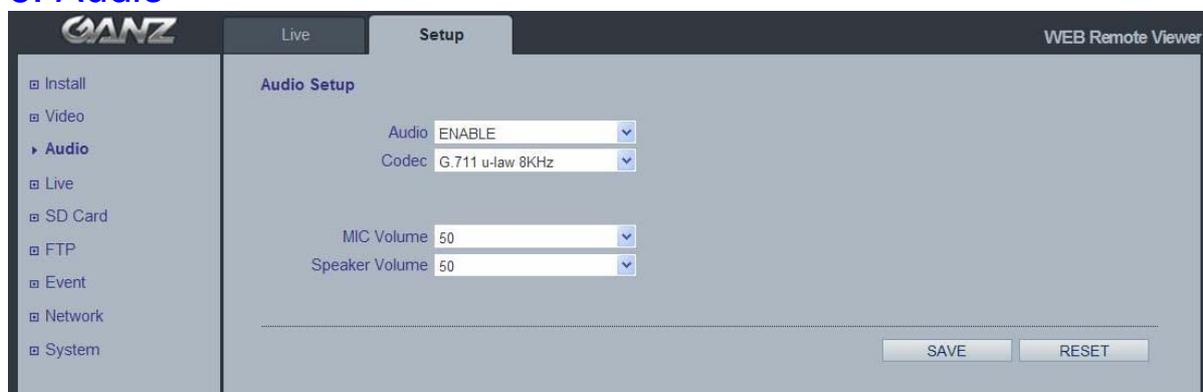
The GANZ ZN-Cx could transmit audio to other clients, using an external microphone and could play audio received from other clients via connected speakers. This section describes how to configure the basic audio settings for the GANZ ZN-Cx, such as setting the communication mode, adjusting the sound levels in the microphone and speakers connected to the camera.
